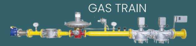
Dual Fuel System delivers fuel gas to the combustion cylinders via the Gas Train into a special Air-Gas Mixer. The mixer is installed on the engine air inlet before the Turbo charger. Combustion is commenced by Diesel as the ignition source and followed by ignition of the GAS MIXER
